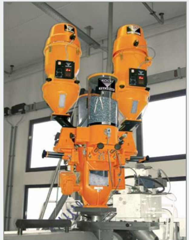
Graviko type GK 150 with dosing stations
