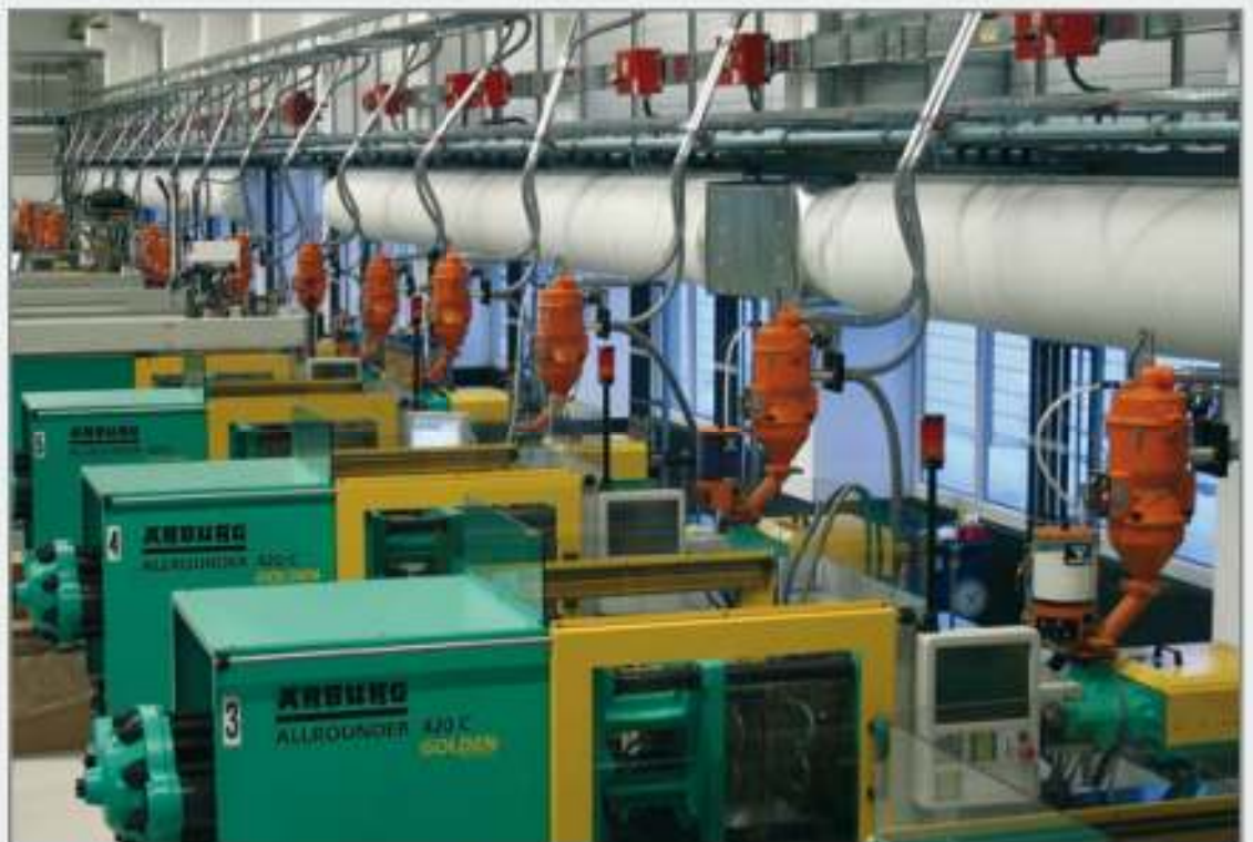
Hopper loaders in combination with KEM units for direct dyeing as modules of a central conveying system.
