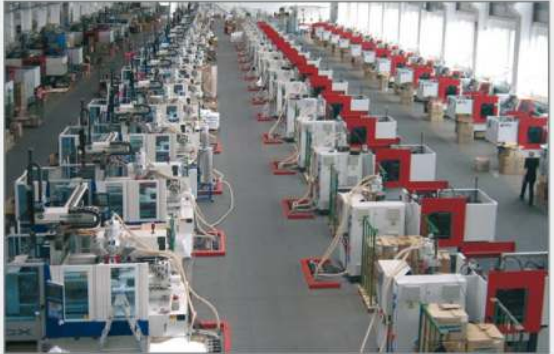
Central conveying system of a toy manufacturer. The conveying system with hopper loaders and drying systems is supplied 108 processing machines.
