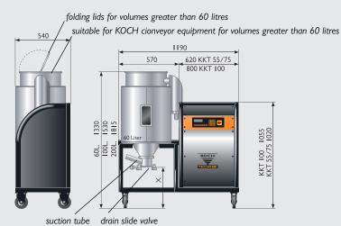
dimension X at 40 / 60 / 100 / 200 litres = 400 mm at 12 + 24 litres = 530 mm
